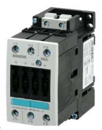
CONTACTOR, AC-3 18,5 KW/400 V, AC 220V 50HZ/240V 60HZ 3-POLE, SIZE S2, SCREW CONNECTION
